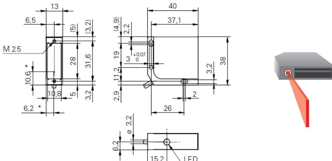
\*optical axis of laser beam
